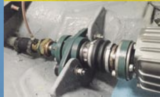
Aquadrive with a Yanmar 2GM engine in a Contessa 32.
