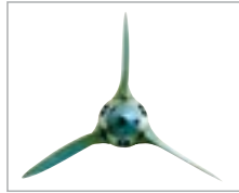
Blades in feathered position for sailing
