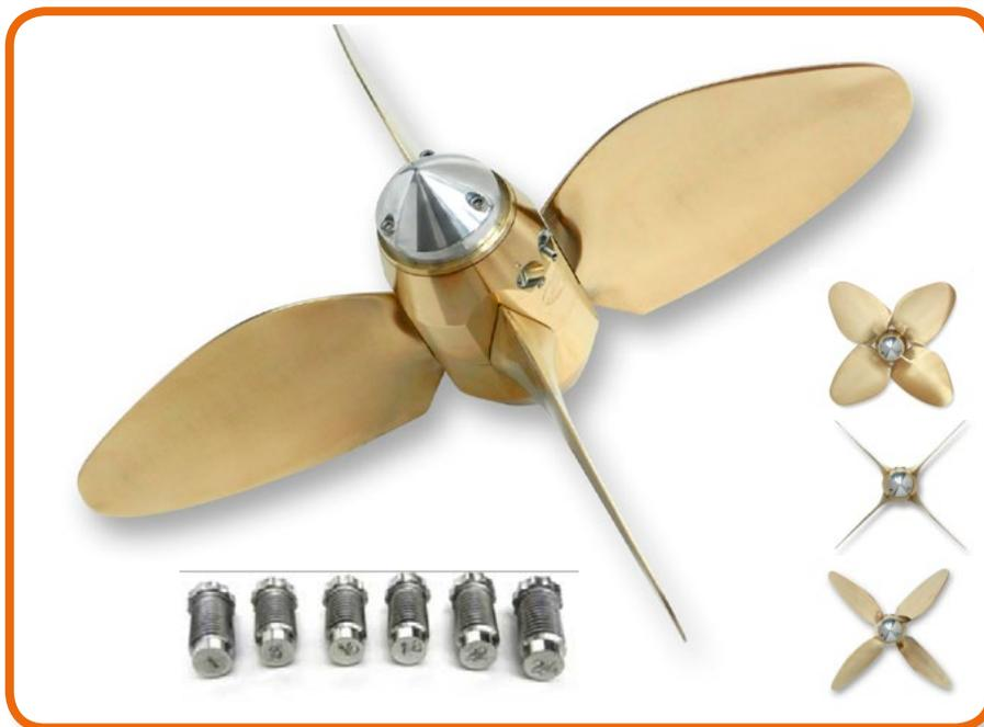
assembled. Just slip the hub on the shaft, secure the nut, lock screws and fit the anode. As with all Max-Prop propellers the Easy model is pitch adjustable. This can be done in the water as the propeller does not need to be disassembled to change the pitch. Should you want to tweak the pitch settings to 'fine tune' your engine loadings you can. Simply swap between pitch screws provided - these alter the pitch in 2 degree increments.
