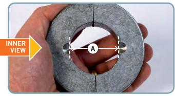
Brand: Max-Prop New code: MP13 (Previous name: Sail drive NOT Rope Cutter) Inner dia 'A' = 45mm (no 'B' dimension required)
