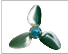
Blades in position for run ahead
